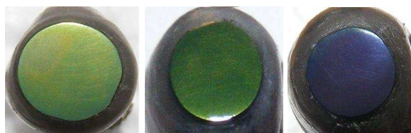
Figure 20. PANI films deposited on the Ni electrode
