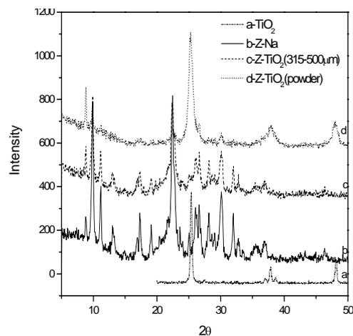
Figure 4. X-Ray diffraction of: a) TiO<sub>2</sub>; b) Z-Na; c) TMZ (315-500 $\mu$ m); d) TMZ (powder)
