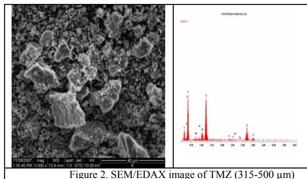
Figure 2. SEM/EDAX image of TMZ (315-500  $\mu$ m)
