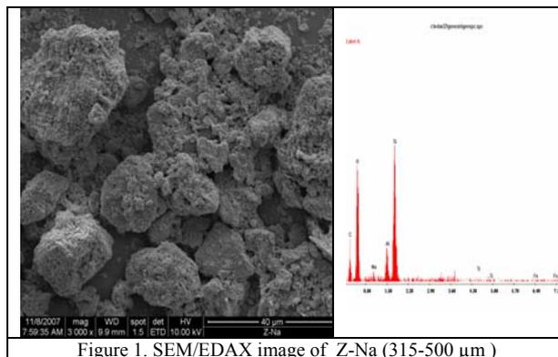
Figure 1. SEM/EDAX image of Z-Na (315-500  $\mu$ m)
