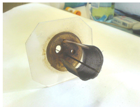
Figure 4. Working electrode block housing the bronze anode and the stainless-steel cathode
