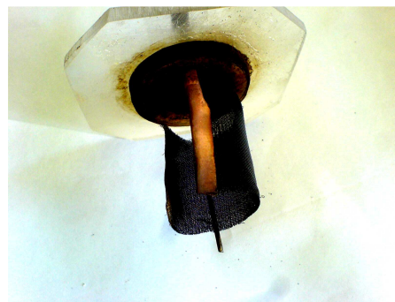
Figure 5. Working electrode block housing the brass anode and the stainless-steel cathode
