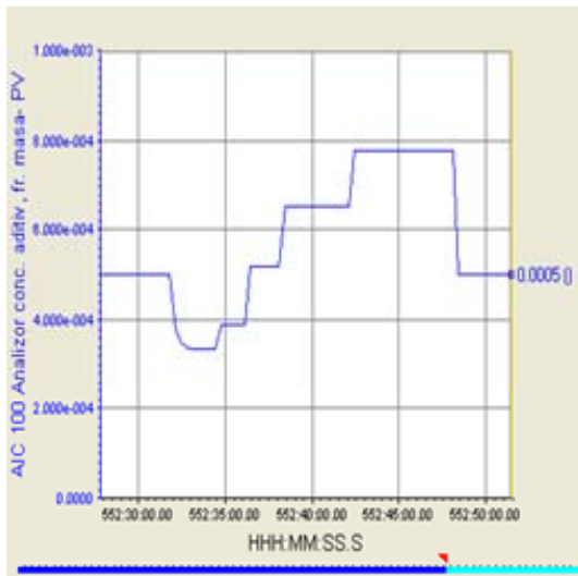
Figure 6. Additive concentration on stream (left side trend) when hydrotreated diesel oil flowrate has a step variation from 50 t/h to 75 t/h (case without ratio controller)
