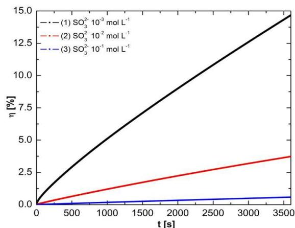
Figure 5. Sulphite electrochemical oxidation process efficiency at  $E=0.65\text{V}/\text{Ag}/\text{AgCl}$
