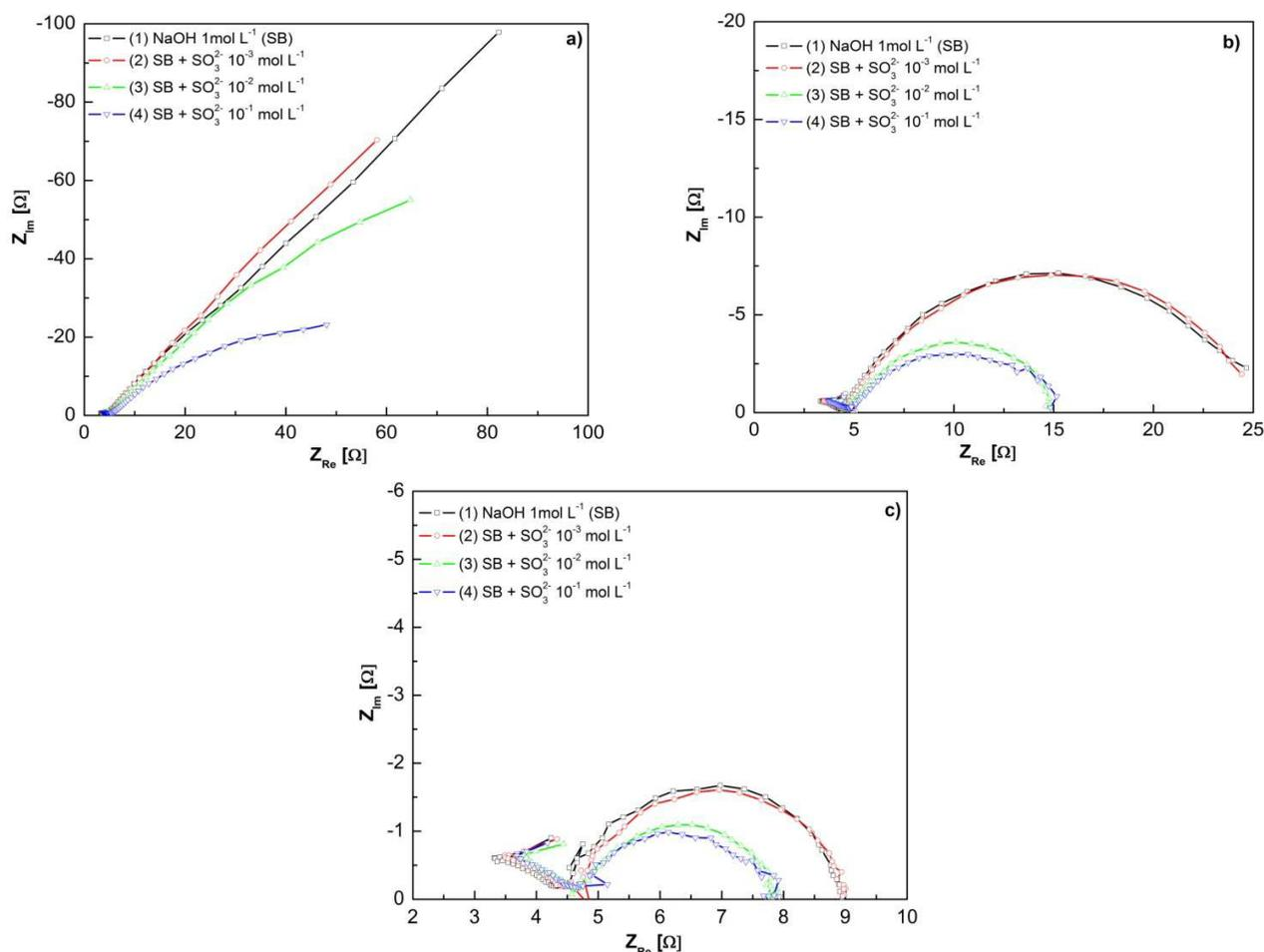
Figure 11. Experimental Nyquist plots recorded for  $\text{SO}_3^{2-}$  anodic oxidation on skeletal electrode in test solutions at different potential values ( $E_{ox}$ ): (a) 0.60V, (b) 0.65V and (c) 0.70V/Ag/AgCl
