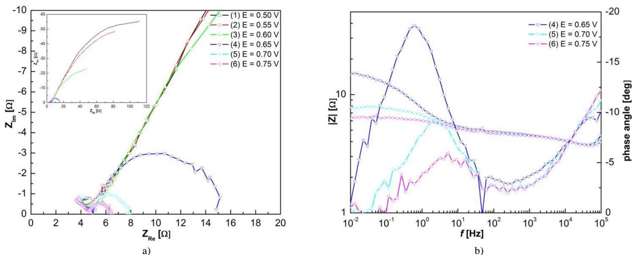
Figure 9. Experimental Nyquist (a) and Bode (b) plots recorded for  $\text{SO}_3^{2-}$  anodic oxidation on skeletal electrode at different potential in  $1 \text{ mol L}^{-1}$  NaOH with  $10^{-1} \text{ mol L}^{-1}$   $\text{Na}_2\text{SO}_3$  solution
