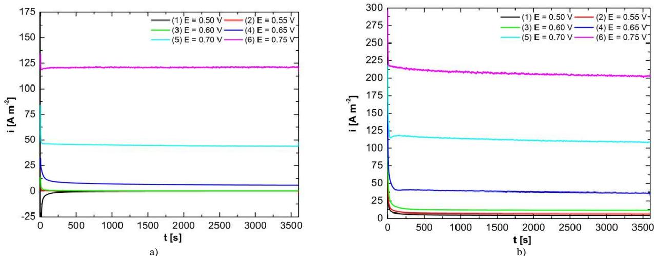
Figure 2. Chronoamperometric measurements on skeletal nickel electrode in  $1 \text{ mol L}^{-1}$  NaOH without (a) and with  $10^{-1} \text{ mol L}^{-1}$   $\text{Na}_2\text{SO}_3$  solution for electrochemical oxidation at different potential values
