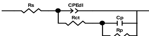
Figure 10. Electrical equivalent circuit used for simulating the impedance spectra of  $\text{SO}_3^{2-}$  oxidation and OER on skeletal nickel electrode in alkaline media
