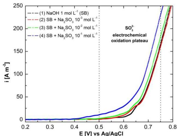
Figure 1. Linear voltammograms recorded on skeletal nickel electrode in  $1 \text{ mol L}^{-1}$  NaOH without/with different concentrations of  $\text{Na}_2\text{SO}_3$  at  $1 \text{ mV s}^{-1}$
