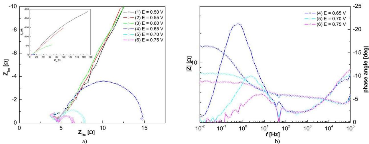
Figure 8. Experimental Nyquist (a) and Bode (b) plots recorded for SO<sub>3</sub><sup>2-</sup> anodic oxidation on skeletal electrode at different potential in 1 mol L<sup>-1</sup> NaOH with 10<sup>-2</sup> mol L<sup>-1</sup> Na<sub>2</sub>SO<sub>3</sub> solution
